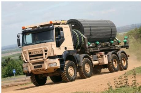
Portable roadway systems allow vehicles to move with ease over difficult terrain conditions such as sand, snow, mud, swamp and ice. As an example, the link given below gives access to a commercially available system.
