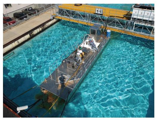
Extreme Spill Technologies designed a new type of oil spill response technology that uses a vessel equipped with a pump system that takes advantage of the oil and water densities to separate the fluids.
