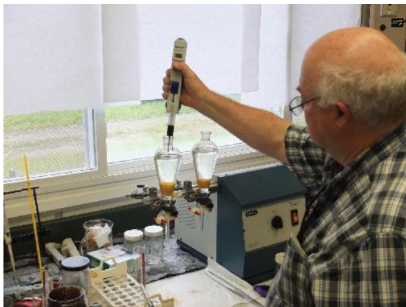
Photo: Ken Trudel of S.L. Ross Environmental Research, Ltd. tests the dispersed oil/water samples in the Ohmsett laboratory.
