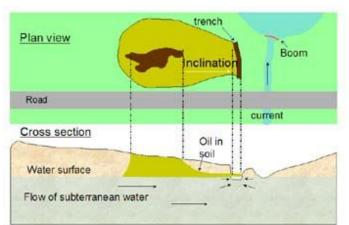
action. In permeable stratum the penetration mainly vertical is whereas in less permeable stratum it is more horizontal. The heterogeneity of the has subsoil а considerable influence on the shape of the penetrating body.
