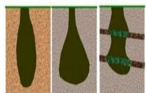
highly permeable less permeable homogeneous soil homogeneous soil
