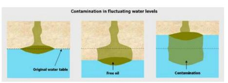
3. The thickness of oil spread out over the water table is not as thick as that measured in the wells.
