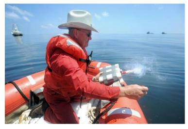
Photo 7 The homemade igniter frequently used during the Deepwater Horizon spill, is lit and prepared to be put into the oil (Photo courtesy of Elastec / American Marine Inc.).
