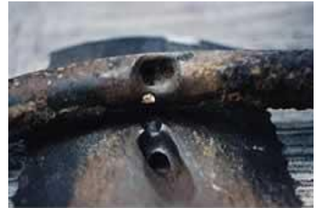
Corrosion and hole in larger gas pipe caused by smaller water pipe on top. Photo courtesy of Jose M. Malo, Electrical Research Institute, Mexico. Source: http://www.corrosion-doctors.org/Localized/sewer.htm ; accessed May 5, 2006.
