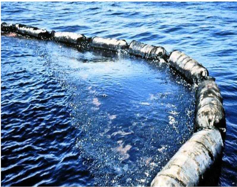
Figure 10 The residue remaining after the first burn of the Newfoundland Offshore Burn Experiment. This is the remains of 50 tons of oil amounting to about 30 kg.
