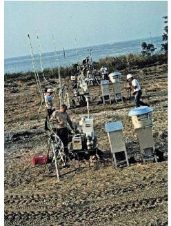
Figure 12 A view of three of the downwind stations used to measure emissions at a diesel burn. Mote than 15 stations were set up with more than 150 instruments. This particular burn was also used to test fire-resistant booms.
