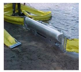
These boom deflectors act like the boom vane but are smaller and fit in between the boom sections, each one drives into the current removing the need for anchors. This is particularly useful in shallow rivers.
