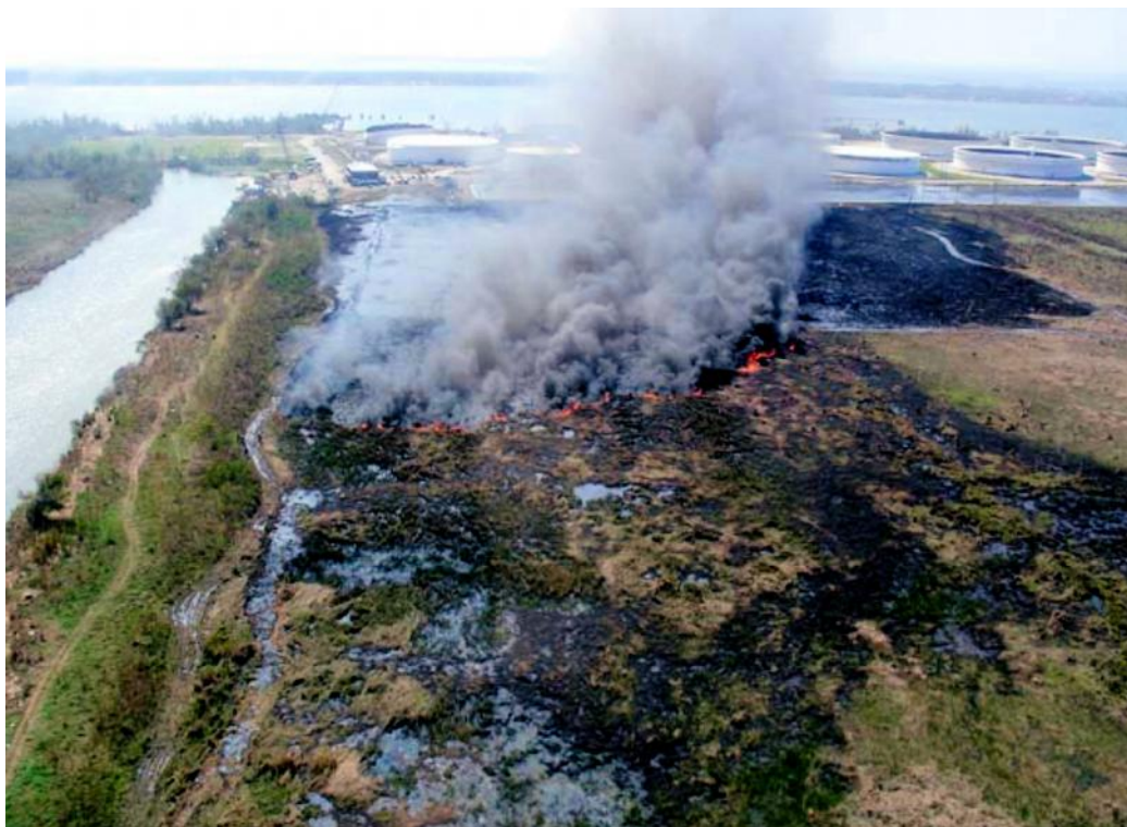
Figure 20 A salt marsh burn in Louisiana. The high water level and topography keeps the fire contained to the oiled area.
