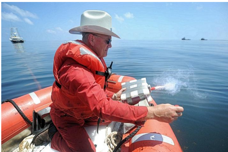
Figure 22 Operator activating an ignition device during the Deepwater Horizon spill. The device consisted of a bottle of gelled diesel fuel and a marine flare. The marine flare melts the bottle and lights the diesel fuel which acts both as primer and burn initiator.
