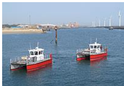
Picture: ALN 122/123 'Elastec III' Wave Skimmer Pollution Control Boats
