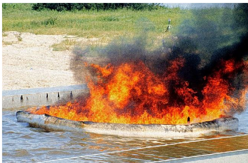
Figure 25 Testing of a fire boom at the USCG Mobile Alabama facility. The testing was done using the ASTM protocol.
