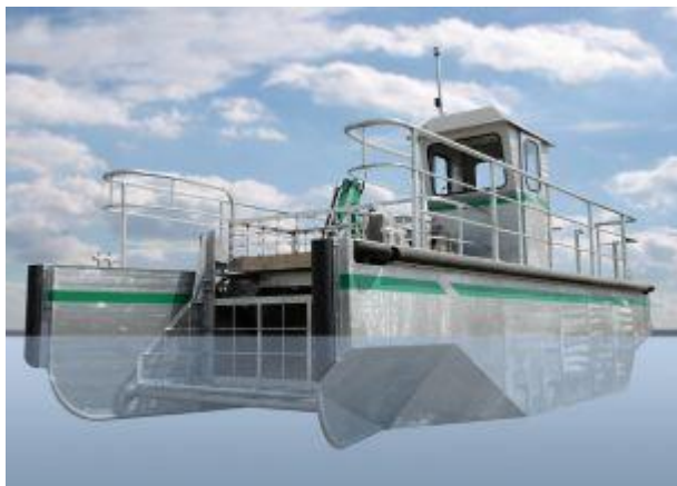
Picture: The 9m floating debris/oil spill collection Envirocat is to be operated by Harbour Clean
