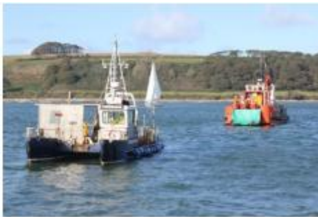
Pictures: MTS vessel Grey Bear deploying the current buster (right) and Pendennis with lines attached assisting (left)
