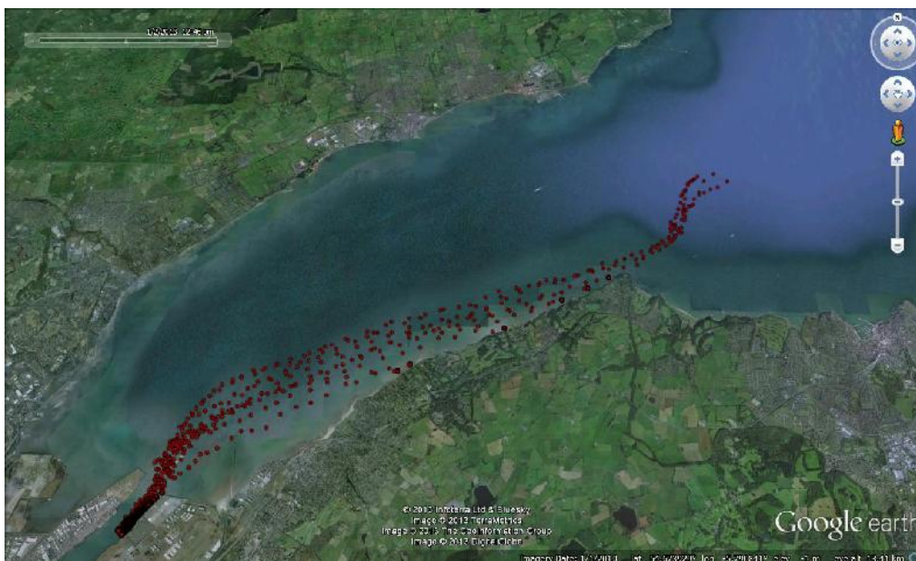
Figure 4. Example of oil spill trajectory from high resolution model in development for Belfast Lough
