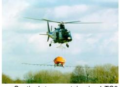
neoprene Shoreguardian boom; 1500 metres of Vikoma Sentinel, two containerised TC3 dispersant systems for helicopter spraying over large areas; and four specially designed 84 kilowatt zone type diesel-hydraulic powerpacks. Vikoma has also carried out specific training for personnel to ensure that a spill response operation can be carried out quickly and efficiently.
