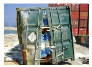
Following a handling accident in a Turkish port, SESMEKE was mobilised in response to two leaking containers. One container contained Diresul, a liquid sulphur dye and the other Toluene diisocyanate (TDI), a very toxic chemical used for the production of flexible polyurethane foam, special varnish and adhesives. TDI can react with water and the humidity in the air to form Hydrogen Cyanide; hence, extreme care was needed in the operation.
