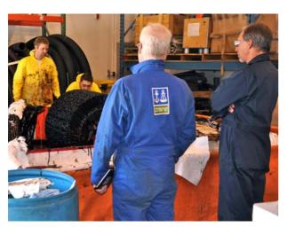
Aqua-Guard recently completed heavy oil testing of their RBS TRITON™ (U.S. Patent 7,303,688) brand of brush oil skimming systems. Tests were conducted to the ASTM F631-99 "Standard Guide for Collecting Skimmer Performance Data in a Controlled Environment" and witnessed by a senior surveyor of Det Norske Veritas, DNV.
