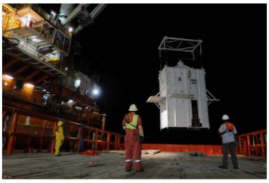
Crewmembers aboard the motor vessel Joe Griffin look on as the mobile offshore drilling unit Q4000 lowers a pollution containment chamber May 6, 2010. The chamber was designed to cap the oil discharge that was a result of the Deepwater Horizon incident. U.S. Coast Guard photo by Petty Officer 3rd Class Patrick Kelley.
