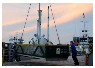
A pollution containment chamber, known as the "top hat", is loaded onto the deck of the motor vessel Gulf Protector at Wild Well Control Inc. in Port Fourchon, La., May 10, 2010. The chamber is the second built by Wild Well Control and will be used in an attempt to contain an oil leak following the mobile offshore drilling unit Deepwater Horizon explosion. U.S. Coast Guard photo by Petty Officer 3rd Class Patrick Kelley.
