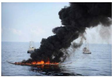
in deploying the fire resistant containment boom and passing it along to shrimp boats whose captains have been trained to tow it during in-situ burns. More info: http://www.elastec.com
