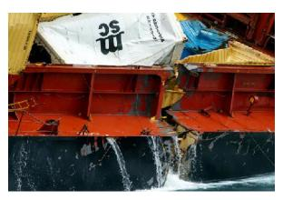
A close-up view of the crack in the Rena's hull. Photo / Katie Cox
