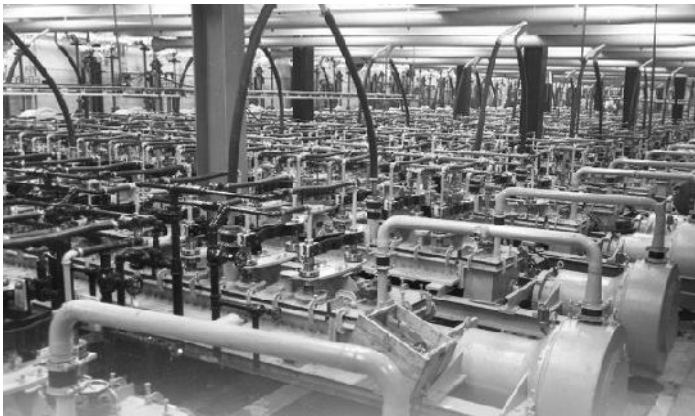
Picture: U.S. Dept of Energy The Colex operation at Y-12 used vast amounts of mercury in the 1950s.
