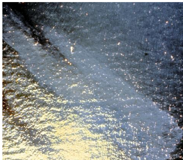
Figure 7 A view of the same test slick (Figure 6) in the visible. The sun glitter makes it difficult to find the edges of the slick
