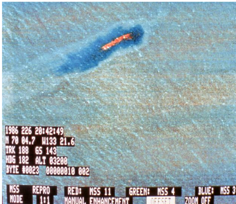
Fig 8 The use of ultraviolet to map thin sheens is shown. The thicker oil is shown in the orange coloration from the infrared. The sheen is in various shades of blue. The outer pale blue fringes are from the ultraviolet which highlights very thin sheen. As there is very little oil in the thin sheens, the UV contribution is not useful operationally.
