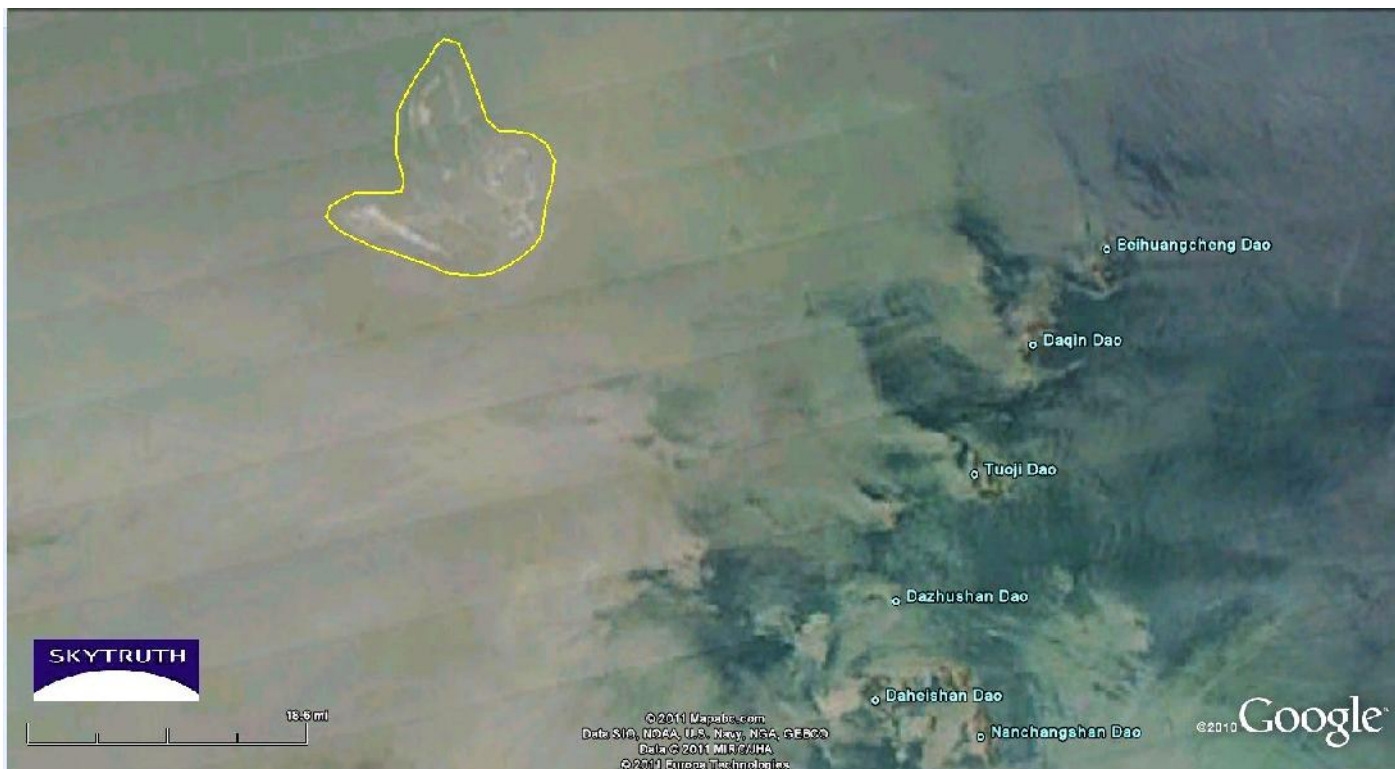
Figure 13 A MODIS image of a spill in China. The MODIS sensor flies aboard the NASA Aqua satellite. MODIS/Aqua image taken June 14, 2011. The oil slick is outlined in yellow. Islands in Bohai Bay are labeled for reference. (Photo from Skytruth website http://blog.skytruth.org )
