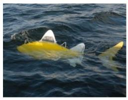
The robots are battery powered and can run for 8 hours between charges (Image: Luke Speller)
