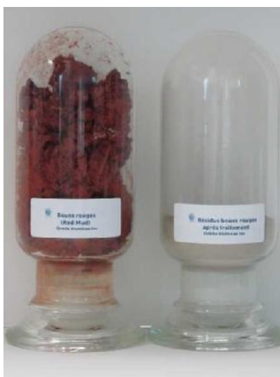
Red mud remediation process; Credit: © Orbite Aluminae On the left, untreated red mud. On the right, sample after treatment.
