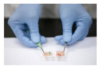
Researchers have developed a special filter coating that essentially can strain oil out of water. It works by repelling oil, but attracting water, which are unconventional properties for a material to have. On an untreated piece of window screen, water (dyed blue) beads up, but oil (dyed pink) soaks through. On the treated surface, the pink oil beads up, but water would soak through. The coating could help advance oil spill clean-up and make it more efficient. Image: Laura Rudic
