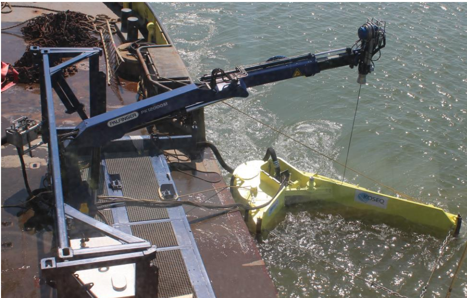
Photo: Compact 502 knuckle boom crane lowers the sweeping arm into the water
