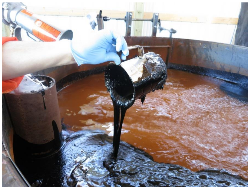
Figure 2 A view of weathered Dilbit showing the viscosity increase after about four days of weathering. The viscosity of the product after spilling slowly returns to the properties of the starting bitumen.
