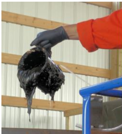
Figure 3 This shows the high viscosity of Dilbit after about 9 days of weathering. The product has largely reverted to the original bitumen by the evaporation of the diluent, condensate in this case.
