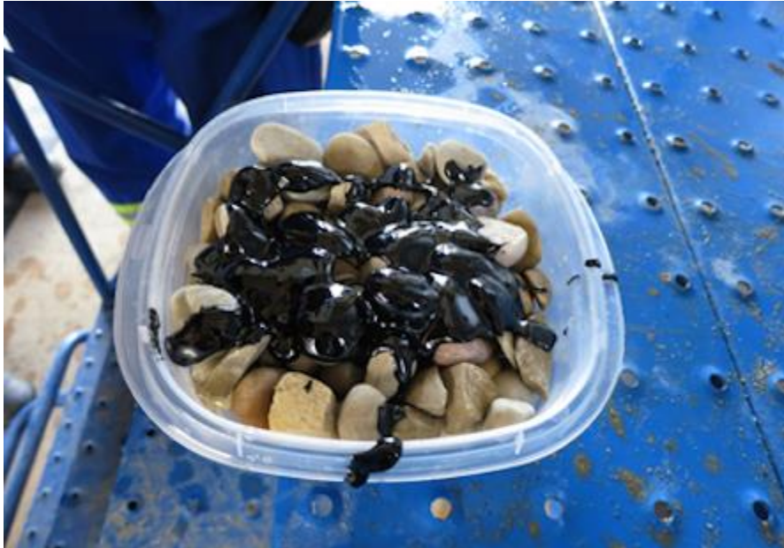
Figure 15 Test of weathered Dilbit gravel penetration – Gainford Tests – May 2013
