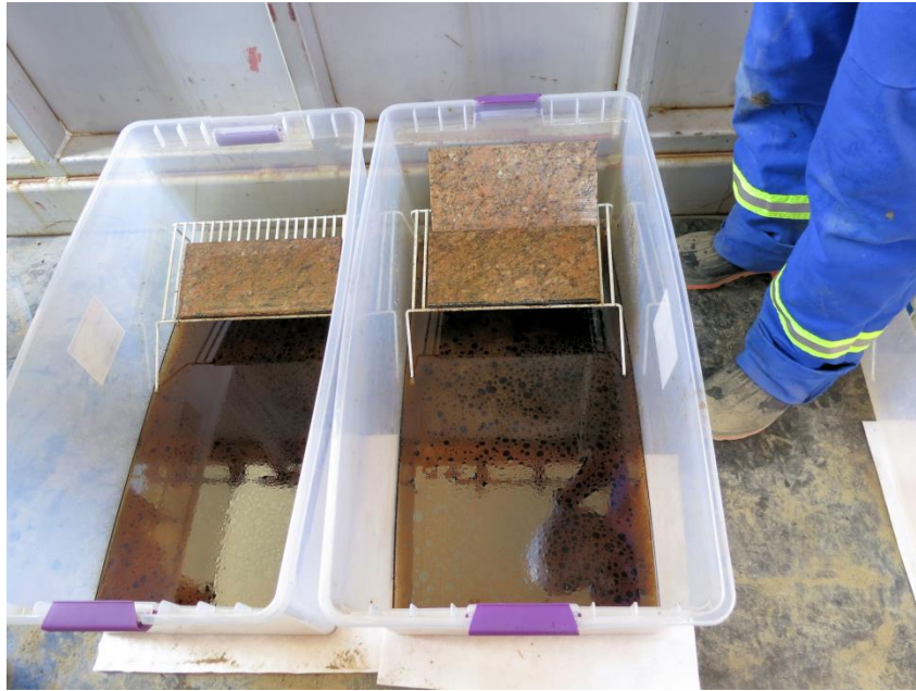
Figure 17 Successful removal of Dilbit weathered for 4 days
