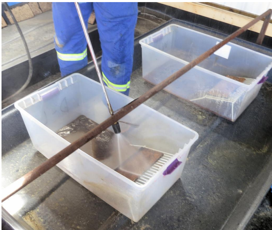
Figure 16 Removal tests of weathered Dilbit from ceramic tokens – Gainford tests, May 2013
