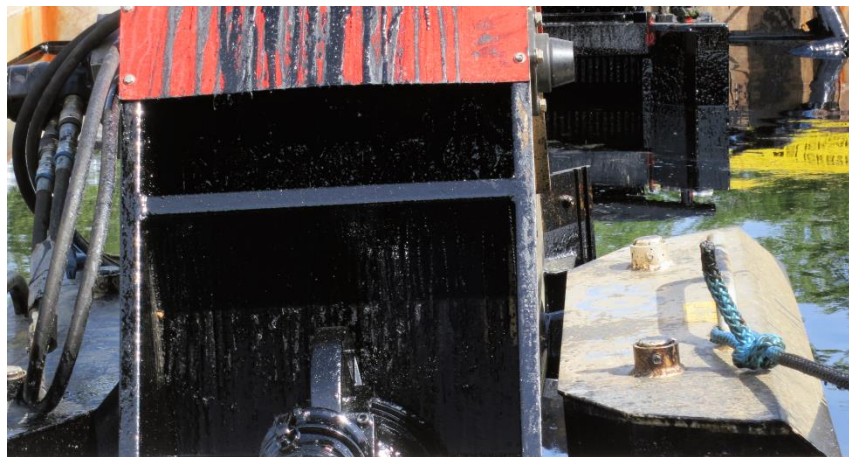
Figure 18 A Lamor skimmer operating during a weathered Dilbit recover test
