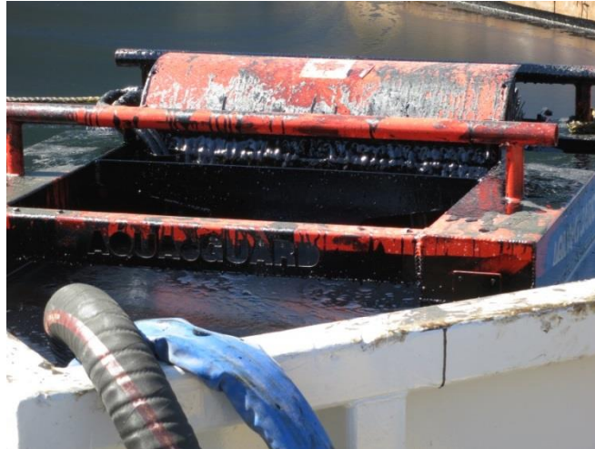
Figure 20 Aqua-Guard Skimmer working at Gainford Trials, May 2013
