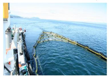
A new oil-spill recovery product makes it easier to clean up spills with just one vessel rather than two, leading to easier, faster and more cost-effective clean-up, according to DESMI, manufacturer of the recovery product.
