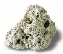
A new patented oil collection method is based on pumice stones from Icelandic volcanic eruptions which occurred thousands of years ago through a very thick ice glacier where the rapid cooling of the Pumice stone (approx. 3.5 cm in diameter) created small air pockets in the stones which made the stone very strong and light plus sufficiently waterproof to keep afloat for up to 5 weeks before sinking. The Pumice is sufficiently resistant to be cleaned and reused within a time spell of 3-5 weeks.
