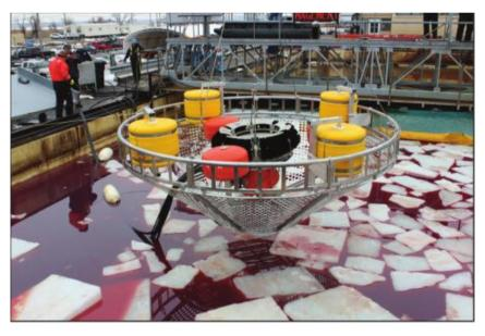
The Desmi Brush skimmer sits inside the ice management system that prevents ice, slush and debris from interfering with the skimmer's ability to pick up oil.
