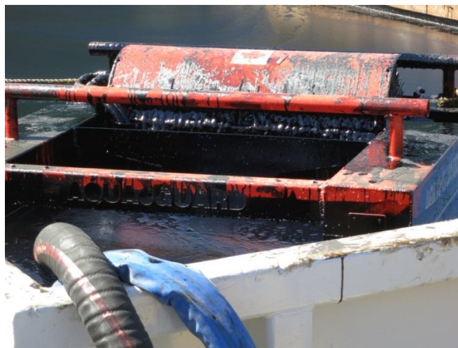
Figure 20 Aqua-Guard Skimmer working at Gainford Trials, May 2013
