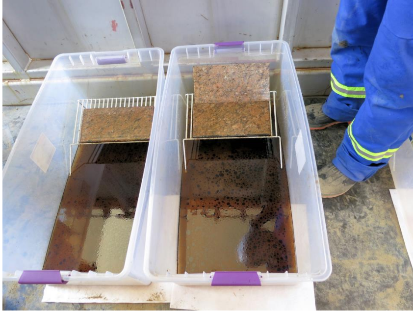
Figure 17 Successful removal of Dilbit weathered for 4 days
