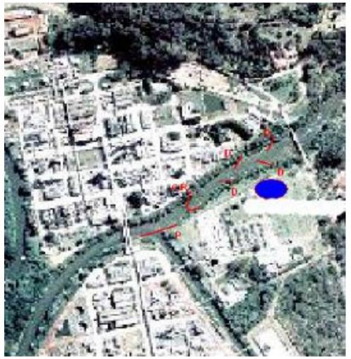
As can be seen the red lines (D) deflect oil into a (CR) U configuration where the apex is in the middle of the river, so recovery will be difficult. In fact oil will be lost.
