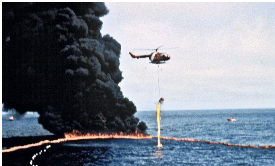
Figure 23 A helicopter discharges remaining fuel from a Helitorch after successful ignition of an oil burn as shown behind the unit.
