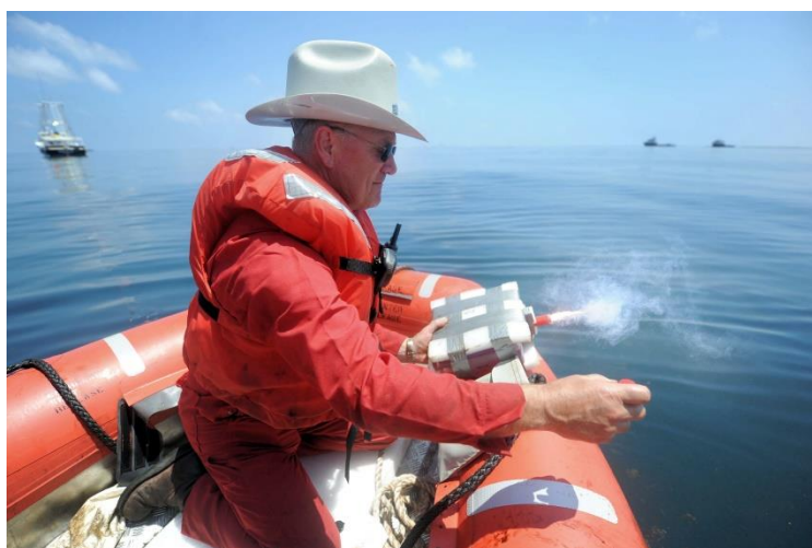
Photo 7 The homemade igniter frequently used during the Deepwater Horizon spill, is lit and prepared to be put into the oil (Photo courtesy of Elastec / American Marine Inc.).
