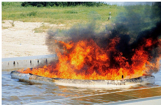
Figure 25 Testing of a fire boom at the USCG Mobile Alabama facility. The testing was done using the ASTM protocol.
