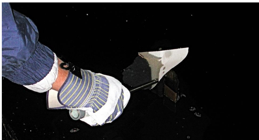
Figure 18 The ignition of a heavy oil. This is easily carried out by adding a small amount of primer such as diesel fuel (about 20 mL), and adding a small wick such as cardboard or paper towel
