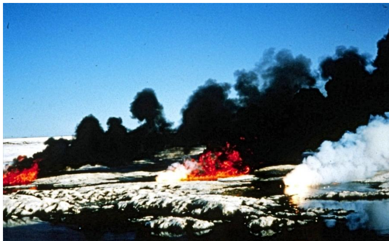
Figure 11 Burning of oil in the Canadian Beaufort. This oil was a test spill put under the ice in the fall. In the spring, the oil resurfaces. The oil was burned as shown here.
