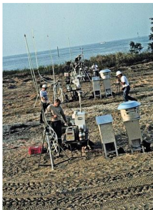
Figure 12 A view of three of the downwind stations used to measure emissions at a diesel burn. Note that 15 stations were set up with more than 150 instruments. This particular burn was also used to test fire-resistant booms.
