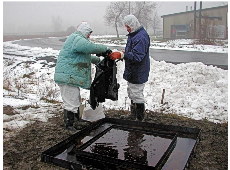
Figure 17 (right) Residue from burning a heavy oil. Note this residue is so solid that it can be removed as a sheet.
