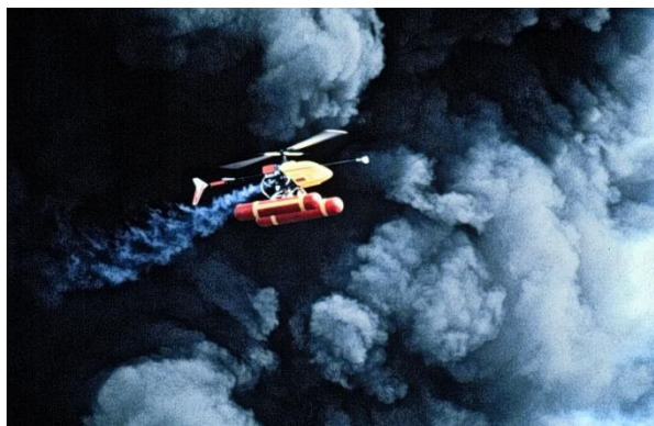
Figure 13 A remote-controlled helicopter emerges from a smoke plume during the Newfoundland Offshore Burn Experiment. Although the most important emissions are measured at ground (1.5 m) level, it is useful to compare these measurements to that in the smoke plume. Many compounds and gases are actually lower in the smoke plume, while the particulate levels (obviously) are very high in the smoke plume.
