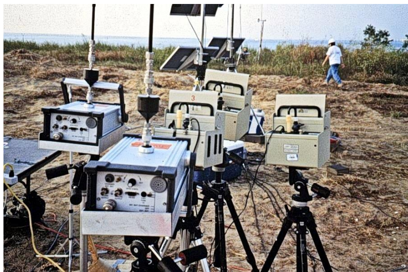
Figure 36 A photograph of a cluster of real-time particulate measuring devices at a burn test site.
