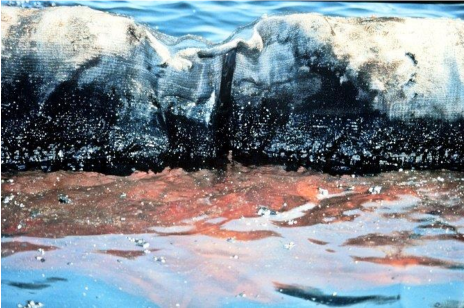
Figure 16 (left) Residue from the second NOBE burn. The residue is dense and as can be seen has a small film of water over it.
