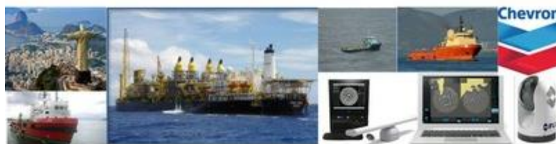
OSD Radars on 3 vessels, additional sensors, Oil Spill Detection, Hydrography SeaDarQ Online with Viewers on the Vessels, the FPSO, central office, authorities Installation in summer 2015
