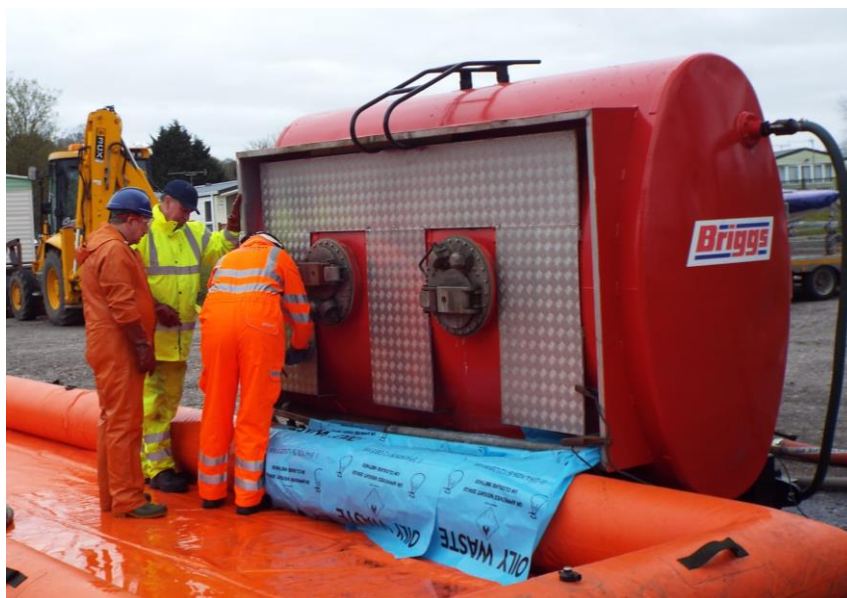
Photo: One-to-one tuition on use of dip tube adaptor for fuel removal from an overturned road tanker. A specially adapted tank barrel is used for training purposes.
