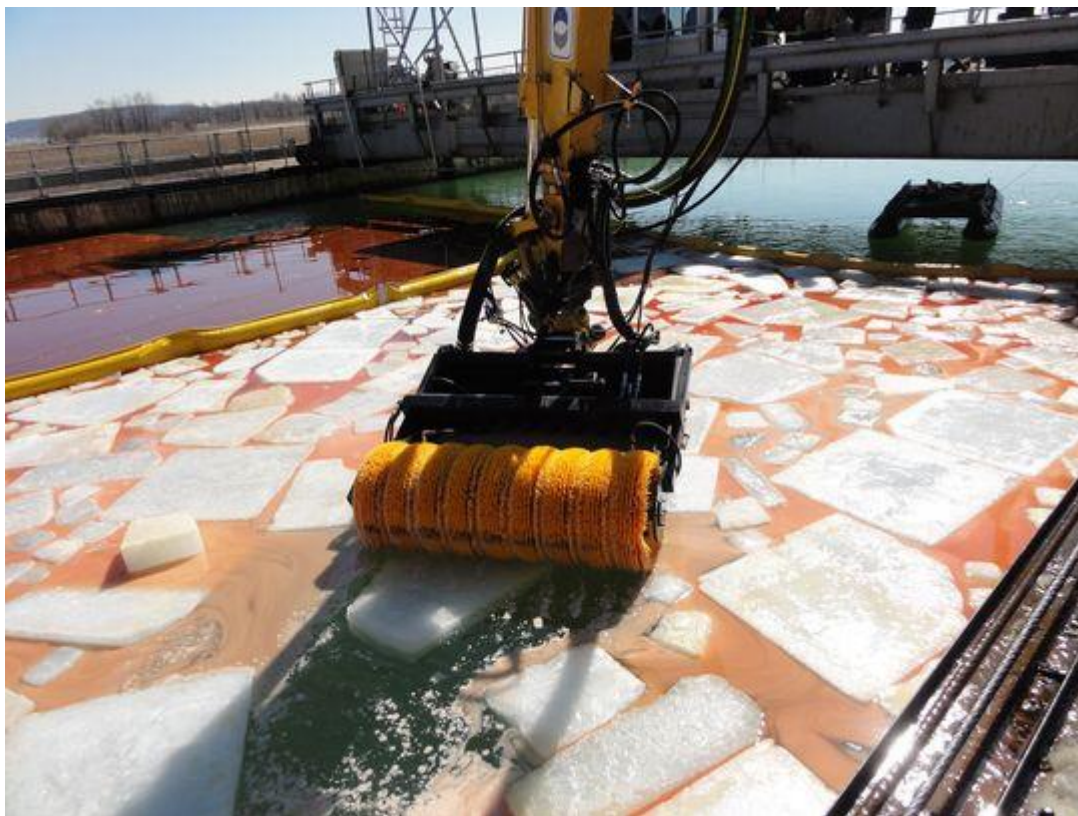
Picture: Placed atop a barge like vessel, a bucket skimmer is moved into place by a mechanical arm such as an excavator. (Photo: Enbridge Energy)
