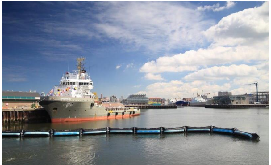
The Ocean Cleanup Foundation's prototype floating barrier sits in front of the MV Union Bear, which later this week will install the prototype in the North Sea. Credit: Ocean Cleanup Foundation.
