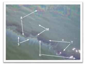
For oil thicker than 50  $\mu$ m the light is being reflected from the oil surface rather than the sea surface (fig 7).
