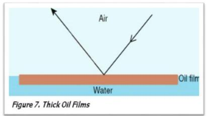
There is no maximum thickness value for True Colours since it is not possible by visual observation from above to estimate the thickness of oil layers above 200 microns.
