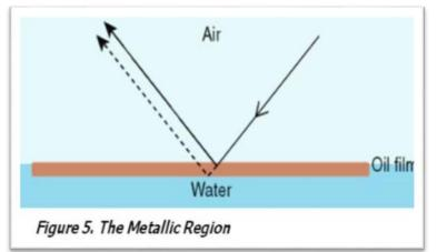
The extent of filtering will depend on the optical density of the oil and the thickness of the oil film.
