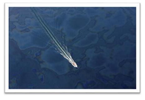
Observers in aircraft, operating at altitudes of 500 ft, 1500 ft or 2500 ft will not be able to see small patches of Code 5 in a background of Code 3, but should be able to see much larger patches of Code 5, perhaps 0.5 to 1 metre across, in a background of Code 3.
