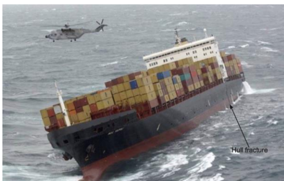
Photo: MSC Napoli after suffering catastrophic hull damage in the English Channel in January 2007. Photo: UK MAIB
