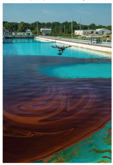
Photo: A rotocraft equipped with a thermal infrared sensor captured images of emulsified oil to validate the sensor's capabilities during the NOAA and BSEE funded remote sensing test.
