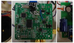
Researchers developed a device that uses florescence from oil (left) to detect its presence and identify the type of oil. The small and simple device incorporates inexpensive electronic components (right). Credit: Oscar Sampedro, Universidade de Vigo.
