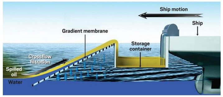
A proposed system for cleaning up oil spills (bottom) modeled after the way filter-feeding fish eat consists of a mesh membrane with pore sizes that get smaller from the bottom to the top. When the membrane is pushed at an angle through an oil slick, a layer of water forms along the membrane, and oil flows over the top into a storage container. The membrane would be attached to a ship for large-scale cleanups. Credit: ACS Nano
