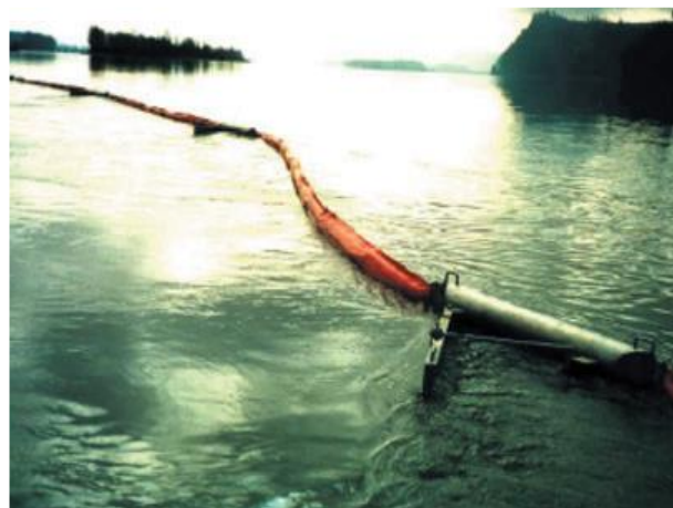
Photos: Below left, booms used to divert oil to a collection point; Below right, a deflector is used to position the boom at the desired angle
