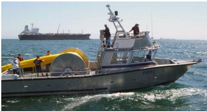
Photo: The 48-foot M/V Duke J operated by the California-based Chevron EL Segundo Refinery has a hydraulic boom reel to deploy and retrieve 1,200 feet of offshore containment boom. Photo courtesy of Chevron El Segundo Refinery.
