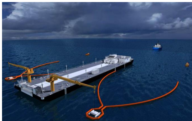
A diagram for an Edison Chouest spill response barge shows an orange boom to corral oil and skimmers suspended off either side to suck up oil. (Photo provided by Alyeska Pipeline)
