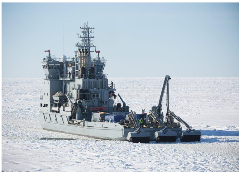
Photo: Heavy duty ice brushes assembled into FNS Louhi, a Finnish multipurpose oil and chemical spill response vessel. Day two of Kemi Arctic 2015 Oil Recovery Exercise and Conference. (Photo courtesy of Jorma Rytkonen/Finnish Environment Institute SYKE)
